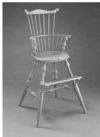
The legs, stretchers and spindles are turned on the lathe. The seat is rough cut on the bandsaw and all the finial shaping and fitting is
